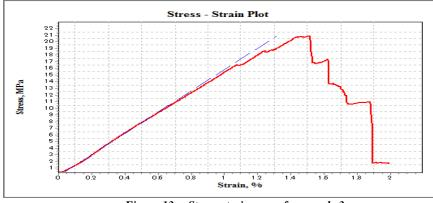
Figure 13: : Stress-strain curve for sample 3
