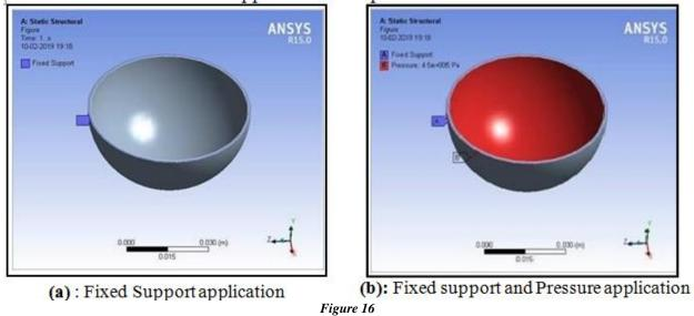
Figure 16(a) shows the selection of the fixed support. The edge is selected as the fixed support. Figure 16(b) shows the combined application of the pressure and the fixed support.
