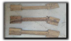
Figure 3: Fractured specimen after UTM testing
